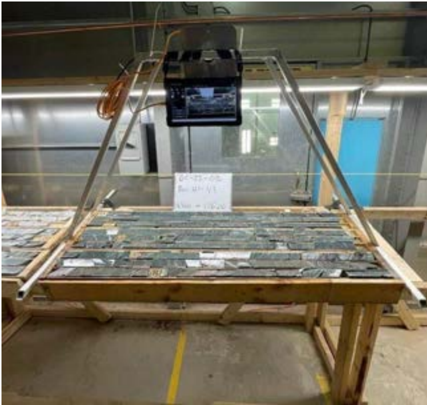
Figure 10.4: Drill core photography set-up with tablet control
