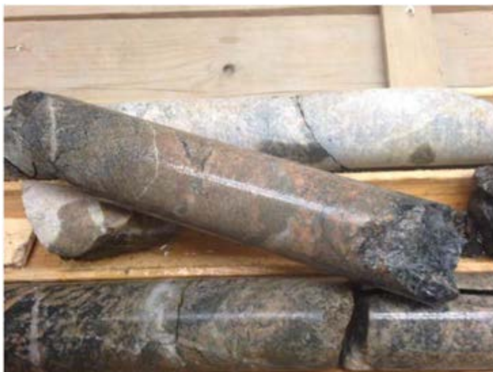
Figure 7.28: Coarse pyrite associated with quartz veined and strongly albitized gabbro from the Stog'er Tight deposit
