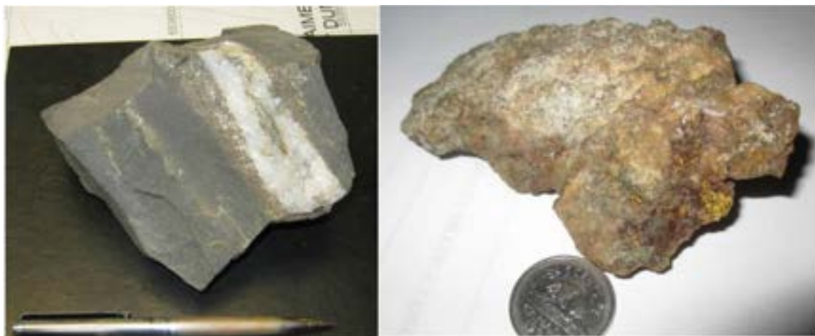
Figure 7.31: Left: Typical ore from the Goldenville prospect. Right: Coarse gold marginal to quartz veining - Deer Cove deposit
