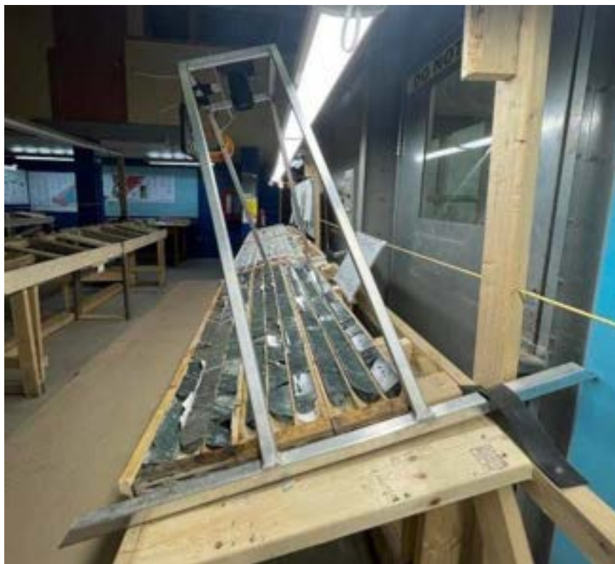
Figure 10.3: Core photography set-up
