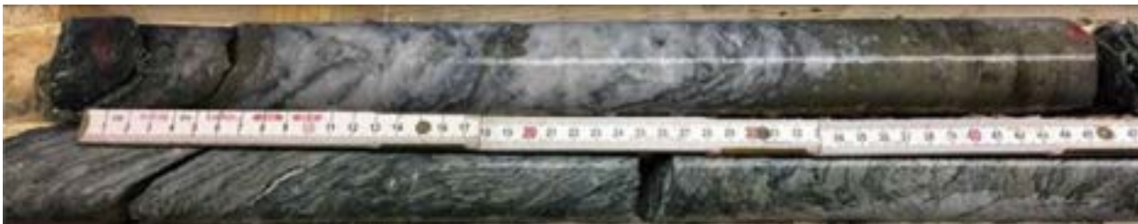
Figure 7.8: Example of veining and mineralization from the Hammerdown deposit
