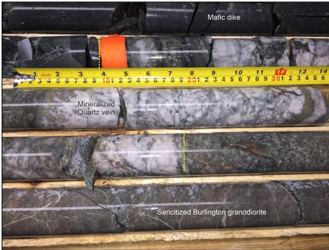
Figure 7.17: Typical mineralization and host rock lithologies at Whisker Valley
