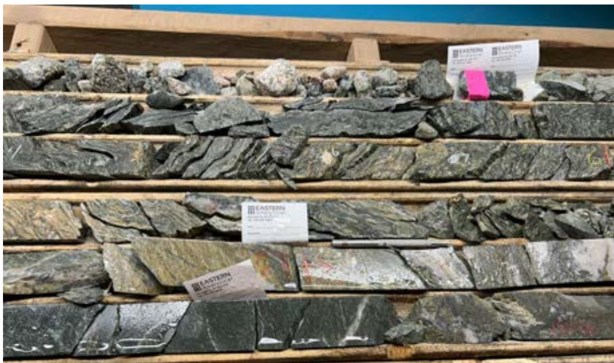
Figure 12.5: Drill hole HDGC-24-038 (8 m depth) showing Wisteria style mineralization
