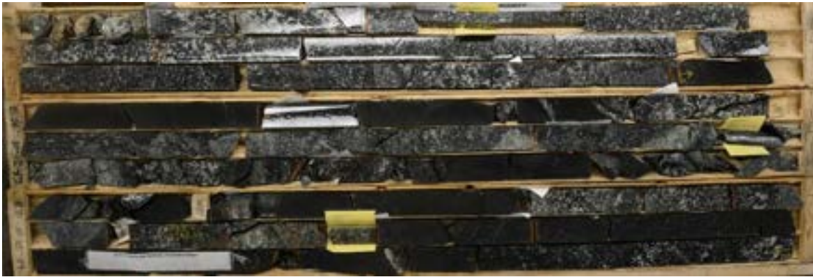
Figure 7.18: Core photograph of the typical alkaline gabbro at Gull Ridge with disseminated pyrrhotite + pentlandite + chalcopyrite ± pyrite
